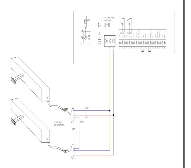
Connection of 2 chain motors to 5A control panel
