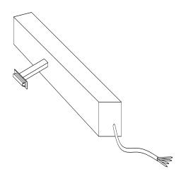
Voltage: 24v D.C. @ 1.5 Amps (see wiring diagram for further info)
