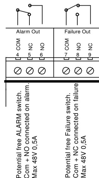
Extra relay print 111655 provides 4 additional potential free switches each 30V 0,5A
